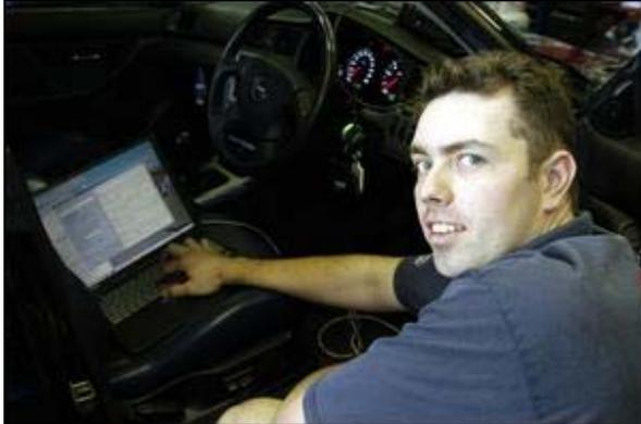
Flashing the new program to the ECU is a 5-minute operation. A laptop (which must contain EcuTeK software) is plugged into the OBD-II connector and the check connector is bridged. Both of these connections are under the dash - there's no need to pull away trim panels to access the ECU.
