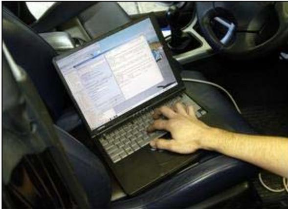
MRT tells us the standard tune in the Australian-spec B4 is very lean and with excessive ignition advance across the rev range. This means the engine is often on the verge of detonation - as many owners can attest to. In a standard or near-standard vehicle, MRT adds extra fuel at wide-open throttle and pulls out 4 or 5 degrees of timing in a number of load/rpm zones.
