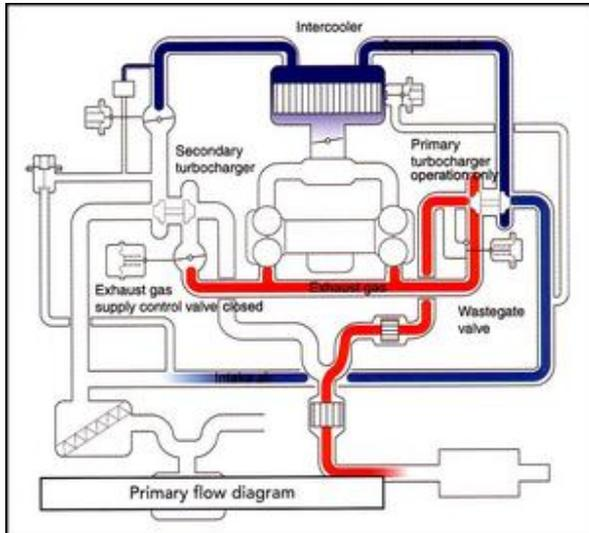
The Subaru B4 employs a sequential twin-turbo arrangement where a relatively small primary turbocharger is used to deliver boost in the low-to-mid rev range. At around 4500 rpm, the sequential control system then begins to feed a proportion of exhaust gas to a secondary turbocharger. Once the secondary turbocharger is spinning fast enough, it provides additional charge-air. In other words, the primary and secondary turbochargers work in parallel at high rpm and load.
