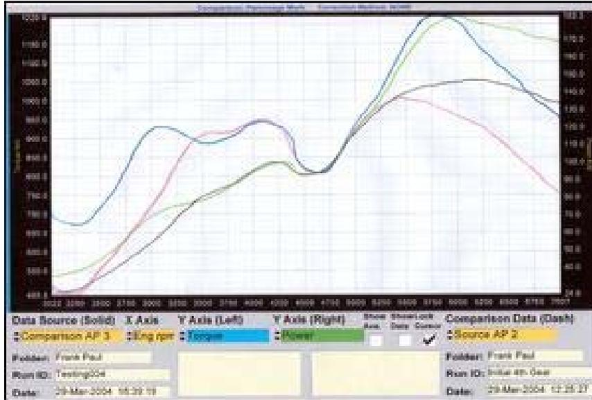
This dyno graph (obtained from MRT's DynaPack hub dyno) shows the gains achieved. The black and red plots represent 'before' power and torque respectively, while the green and blue plots represent the 'after' power and torque curves. Each run was conducted in fourth gear. As you can see, torque is increased by a massive 30 percent at just 3000 rpm. At the top of the rev range, peak power has been elevated from 150 to 183kW at around 6000 rpm. That's a 32 percent gain.
