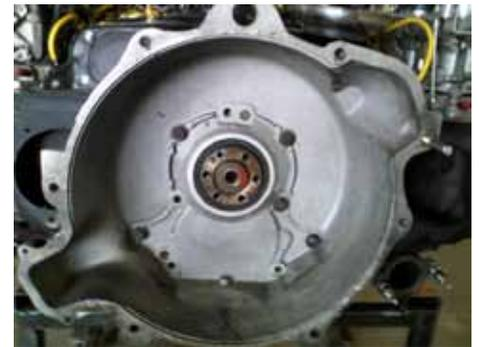
**No wonder it leaked oil, four missing bolts. The ones that were there were loose, plus a missing gasket.**
