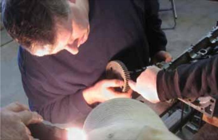
**Greg Renfro got a lot of help locating the timing mark on the cam gear for the engine he was assembling.**
