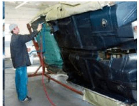
Applying "lizard" undercoating to a freshly prepped undercarriage
