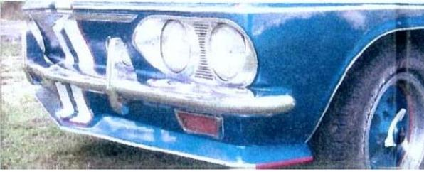
**FIFTH:** Since I had blended the rear spoiler in with the hood, Def. #5 struck took over again. I enclosed the underside of the spoiler end that extended over the rear fenders, and covered it with a strip of reflective tape. On my trip to California, that paid off when a tow truck driver I was waiting for almost missed me in the dark.
