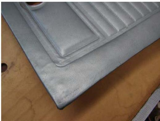
Be sure and remove any burrs from cutting the sheet metal, and make sure to form the sheet metal so the edges curve toward the cardboard you are gluing it to, so you don't have any edges showing through the vinyl when you are done.
