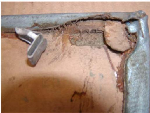
What do you do when you remove a door panel carefully and it still pulls the clip out of the door panel?
