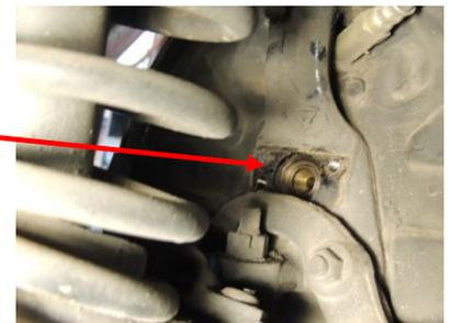
14. Insert the end of the cable in the hole on the dust cap and gently tap the cap back on the hub. Use the raised edge of the cap to tap on,
