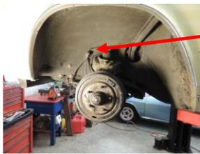
7. Take the bracket loose that holds the cable to in the wheel well.
