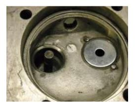
After the set screws have been cut off they are ground flush with the cylinder head. If done carefully the valve seat surface will not be disturbed.
