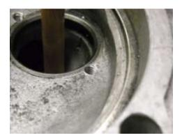
Set screws with high temp adhesive have been tightened into those holes.
