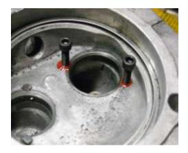
A Dremel tool was used to cut off the set screws. A washer protected the valve seat during cutting. Set screws next to the exhaust valve seat were cut off too.
