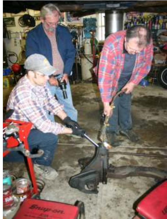
Used the torch a couple times to loosen things up a bit.
