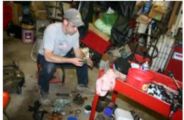
Bill Jr. packing wheel bearings.
