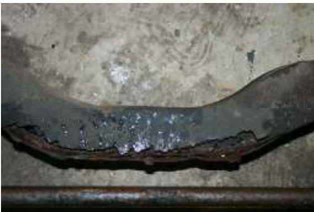
The 68-69 suspension is especially prone to the dreaded tin worm eating away at it due to an extra shield installed to protect the suspension that only made matters worse! Here is a close up so you know why we replaced the front cross member.
