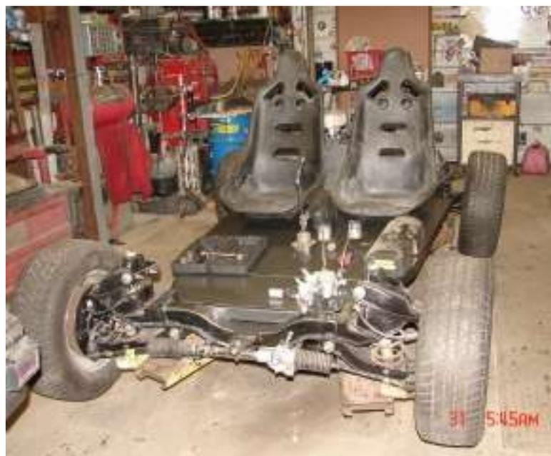
“The front hubs came from an LM Corvaire. It also has a hydraulic clutch and a Line Lock roll
