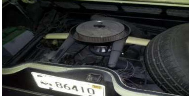
The late model convertible always looked terrific and in this light color, especially entertaining. To my dismay it had the s-l-o-w Powerglide 2-speed transmission and an aftermarket Edelbrock 4-barrel carb [instead of the 4-carb 140 hp setup implied by the air cleaner].
